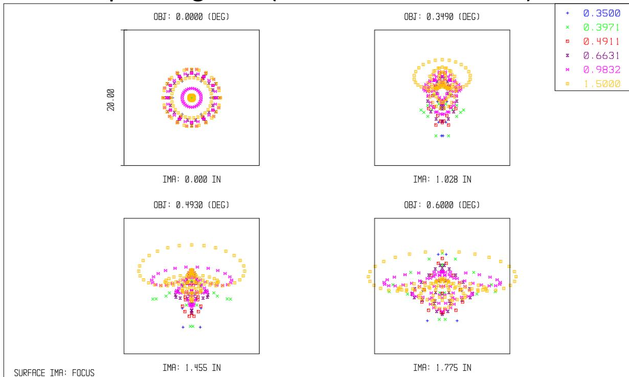
Geometrical Spot Diagrams 6 colors and 4 field angles (Does not include diffraction)
