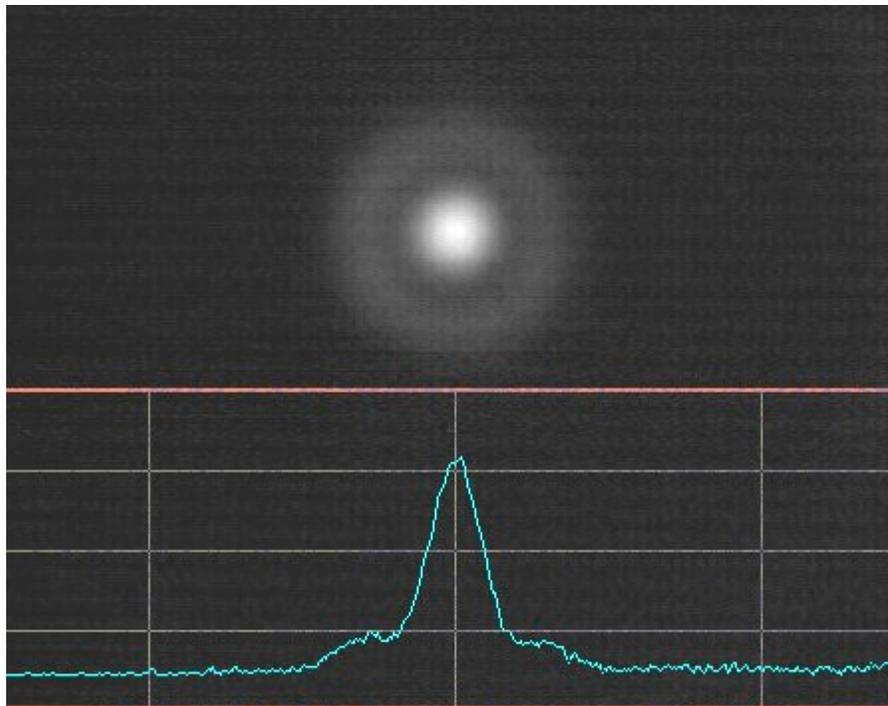
Actual Airy disk of an unobstructed aperture with an intensity scan through the center in blue.
